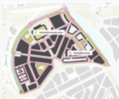
Gray: Separated sewer and permeable pavement
